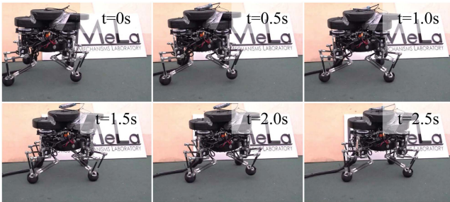
Fig. 24. SCALAR three-DoF leg walking configuration with a 14.7-kg payload, equivalent to 233 % of its weight.
